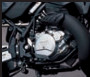
MX 14 Engine >> single-cylinder, two-stroke, liquid cooled, environmentally-friendly
