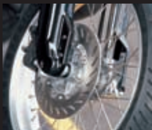
MX 13 Front brake: >> disk, 230 mm dia., floating calliper, double parallel piston
